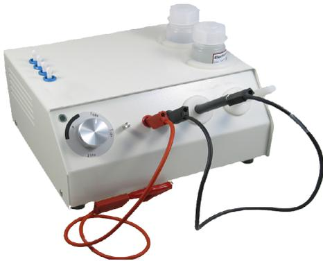
This optional device can be used for easy conversion of existing microsection labs, which still operate with aggressive chemicals, to an electrolyte process. The station is used for the **preparation of polished surfaces** after cutting and polishing the sample. A felt tip dipped in electrolyte is used as the cathode in this case. It removes the burrs and prepares the microstructure so that the relevant details can be seen.
