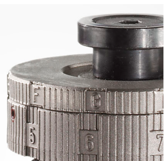
crimp height adjustment
