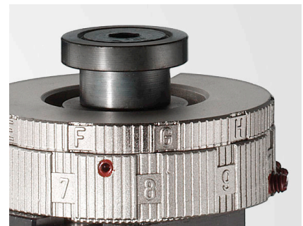
crimp height adjustment
